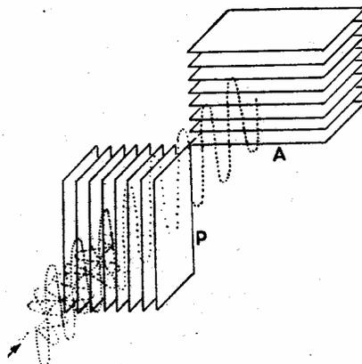
Figure 2: One of mutual positions of a polarizer and an analyzer
