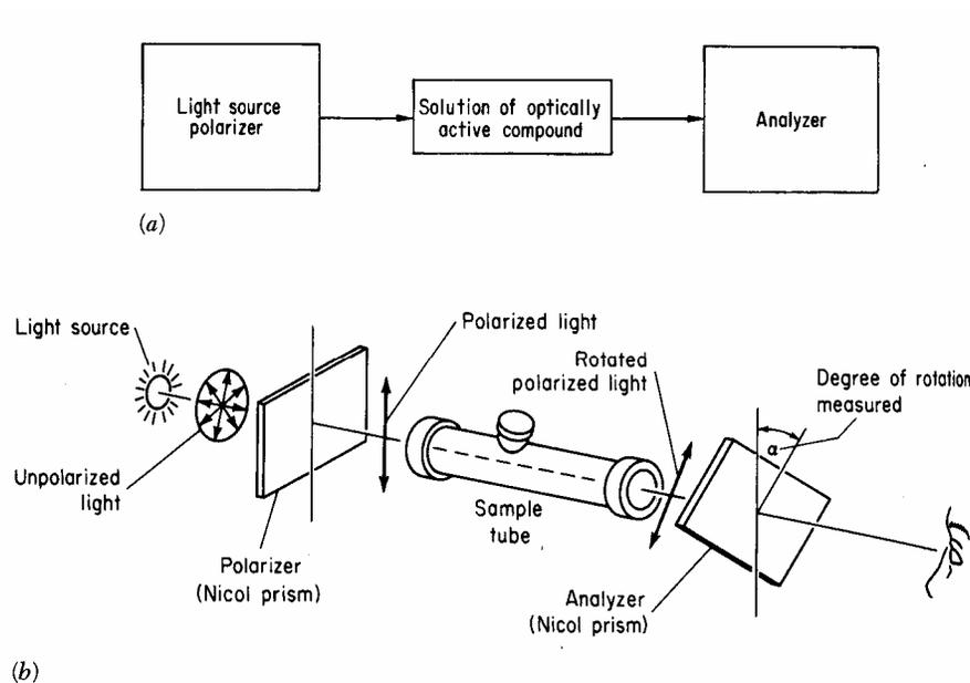
Figure 1: a) principle of a polarimeter set up
